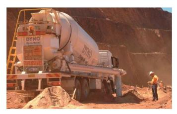
These explosives are based on high ratios of emulsion to ammonium nitrate prill, which promote a physical barrier between the prill and the reactive ground.
